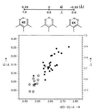
Figure 22. Resonance-assisted hydrogen bonding (RAHB) in enolones according to Gilli et al. [114] The parameter Q measuring the degree of  $\pi$  delocalization decreases with decreasing  $O \cdots O$  distance (Q=0 indicates a completely delocalized  $\pi$  system). Stars represent intramolecular, and squares represent intermolecular hydrogen bonds.
