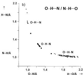
Figure 14. Lengthening of the X–H bond in X–H ··· A hydrogen bonds. a) Correlation of O–H and H ··· O distances in O–H ··· O hydrogen bonds. [92] The plot is symmetrized with respect to the two O atoms. [31b] b) Correlation of N–H with H ··· O bond lengths and O–H with H ··· N bond lengths. [93] The right branch shows N–H ··· O, and the left branch O–H ··· N hydrogen bonds. Both plots are based on neutron diffraction data.
