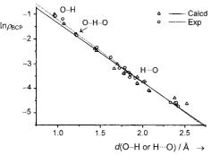
Figure 3. Electron density at the bond critical points,  $\rho_{BCP}$ , for a set of O–H···O hydrogen bonds, together with fitted logarithmic relationships for experimental and theoretical data. (Adapted from ref. [41].)
