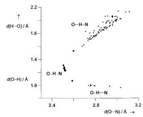
Figure 15. Correlation of O–H and H  $\cdots$  O bond lengths with the O  $\cdots$  N distance in O/N–H  $\cdots$  N/O hydrogen bonds (neutron diffraction data). [93]
