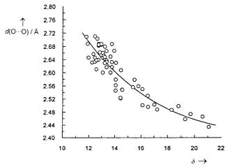
Figure 5. Typical correlation of  ${}^{1}H$  NMR chemical shift and  $O\cdots O$  distance in  $O-H\cdots O$  hydrogen bonds. [56c] Other authors have obtained similar figures from different structure samples. [6, 56a,b]
