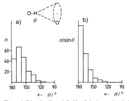
Figure 6. Directionality of O–H···O hydrogen bonds in carbohydrates (H···O < 2.0 Å). a) Conventional histogram with a maximum at slightly bent angles  $\theta$ . b) Histogram after "cone correction" (weighting with  $1/\sin\theta$ ) which represents the frequency of H-bonds per solid angle. [59] Angular preferences can be seen properly only after cone correction.
