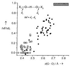
Figure 18. Effect of C–O–H···O=C hydrogen bonding on C $\sim$ O bond lengths. The quantity  $\Delta d$  is the difference between the donor C–O and the acceptor O=C bond length ( $d_0$ =value for fragments free of hydrogen bonding; squares: combination of acid and complementary base; dots: resonance-assisted hydrogen bonds). [46]
