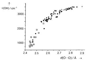
Figure 4. Scatter plot of IR stretching frequencies  $\tilde{v}_{OH}$  against  $O\cdots O$  distances in  $O-H\cdots O$  hydrogen bonds (squares: combination of acid and complementary base; filled circles: resonance-assisted hydrogen bonds (RAHB); triangles:  $\sigma$ -cooperative hydrogen bonds; crosses: isolated hydrogen bonds). [46] (IR data from ref. [45a].)
