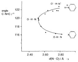
Figure 20. Effect of hydrogen bonding on the C-N=C angle in pyridine.[10f]
