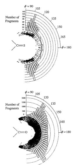
Figure 9. Acceptor directionality of C=O (bottom) and C=S (top) groups in N/O–H···O/S=C hydrogen bonds.  $^{[69]}$  Note that the directionality is much more blurred for C=O than for C=S.
