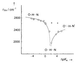
Figure 25. Correlation of  $\Delta p K_a$  and the IR stretching frequency of crystalline pentachlorophenol-amine adducts. The symbols  $\times$  indicate outliers, presumably caused by crystal-field effects. Very strong hydrogen bonds occur only in a certain "critical" region of  $\Delta p K_a$  values.[104a]
