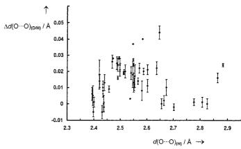
Figure 21. H/D isotope effect on hydrogen bond lengths. The difference of  $O\cdots O$  distances in pairs of D and H compounds is plotted against the  $O\cdots O$  distance of the H compound. A value of  $\Delta>0$  means that the hydrogen bond in the D compound is longer. [108]
