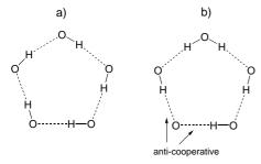
Scheme 16. Cycles of five hydrogen bonds.<sup>[119]</sup> In the preferred "homodromic" arrangement (a) all hydrogen bonds run in the same direction. In the less common "antidromic" arrangement (b) a change of orientation leads to local anticooperativity.
